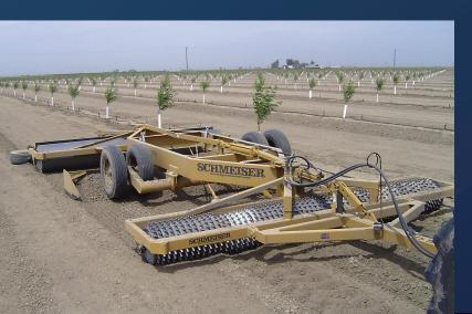
The wheel transport is operated by a single hydraulic cylinder, which lifts the unit high off the ground for easy transport. It is also equipped with positive rod control steering locks for operating on highways.
