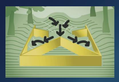
The idea is simple. First, the "V" Blade Leveler slices and crowds dirt to the center, then it pushes dirt back towards the outside (continuously cutting and filling). The rear smoothing plate or the roller model act as a stabilizer to firm and flatten the soil as well. The reversible cutting blades are curved, so dirt, trash and vegetation is sliced and rolled (like a roadgrader blade). Blade mounts are slotted so cutting depth can be adjusted.
