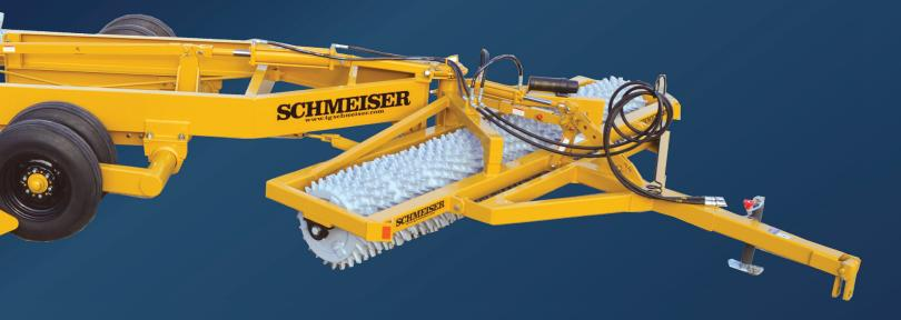
The front roller section is equipped with a Till an' Pak unit that breaks clods and pulverizes the soil. The center section has a heavy duty bucket that fills holes and levels. The rear section is equipped with a 20" diameter Smooth an' Roll unit. Water can be added to both front and rear rollers for additional weight.
